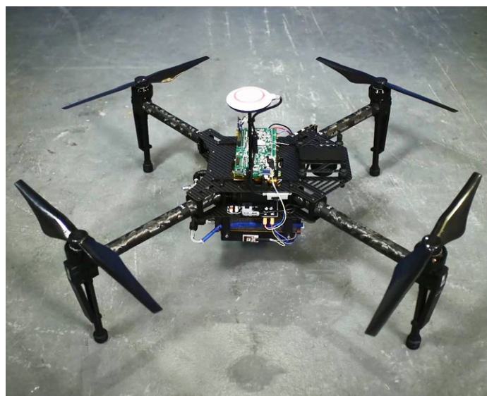
A drone prototype equipped with a fuel cell stack from Intelligent Energy.
