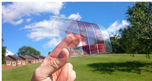
Flexible solar cell. Source: University of Surrey
